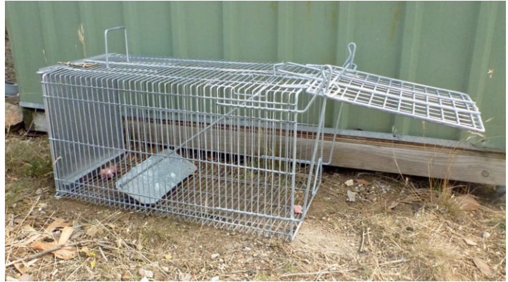
'Treadle-style' cage trap with a lure tied at the back and a small 'taster' at the front. Photo courtesy of Sue Robinson DPIPW.
