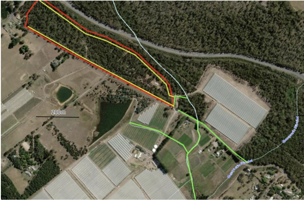
Figure 7 Existing drains (green lines) and proposed new drains (yellow lines) on the development area (outlined in red) and adjacent property (as 105 Hillwood Road) and waterways present (blue line)
