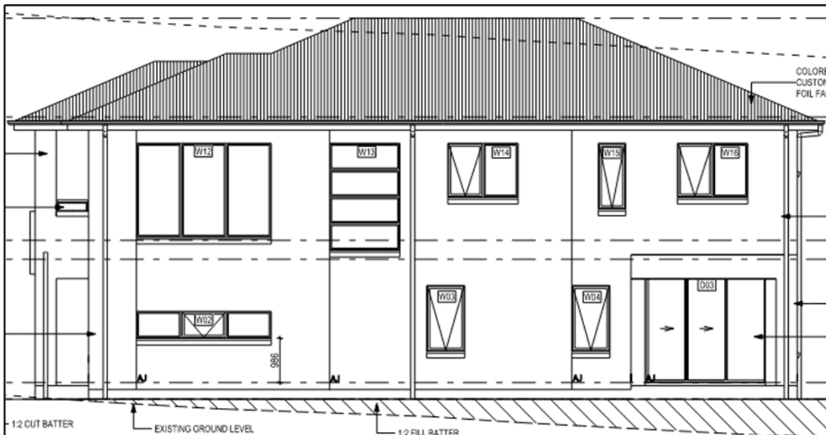
Figure 8: Elevations - Western Elevation
