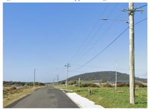
North Street has a seal width of 6m and should be widened to support growing function as an Urban Collector Road.
