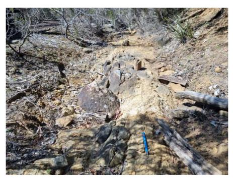
Photo 18. Highly weathered dolerite bedrock exposed in washed out access road, joints dipping steeply ~85° towards 060° (northeast), looking southeast.
