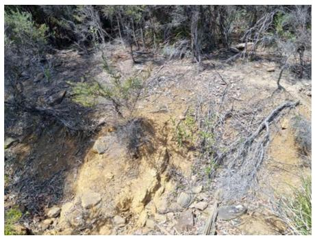
Photo 15. Highly weathered dolerite bedrock exposed in road cutting, overlain by  $\sim$ 0.2-0.3m of colluvium. Joints steeply dipping  $\sim$ 85° towards 140° (southeast), looking southwest.
