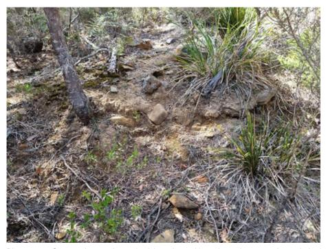
Photo 13. Orange brown low plasticity clay with subangular to subrounded dolerite cobbles/boulders (possible colluvium derived from Jurassic-aged dolerite) in ~1m high road cutting, looking west.
